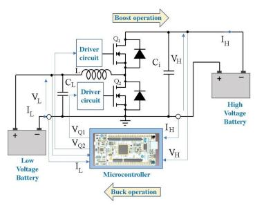
the testing and control of a half-Bridge board with SiC devices to evaluate the operation of a Buck and Boost type topology typical of non-isolated bidirectional battery chargers. The thesis foresees the analysis of the topology, through simulations, the development of a control (current and voltage to follow a charger profile) and the implementation of the control method by means of an actual microcontroller (Nucleo STM32) and relative operation tests.
