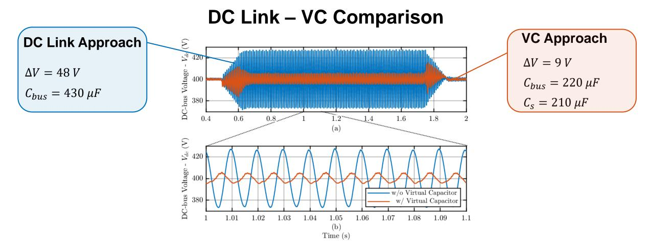
80% reduction of the ripple at steady state with the same total capacitance
