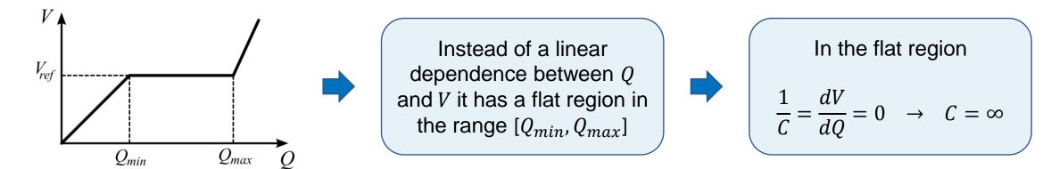
It is possible to try to emulate this behavior by means of an auxiliary circuit connected to the DC bus
